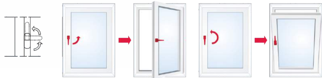
Turn and tilt window (closing - turning - tilting)
