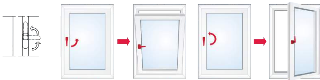
Tilt and turn window (closing - tilting - turning)
